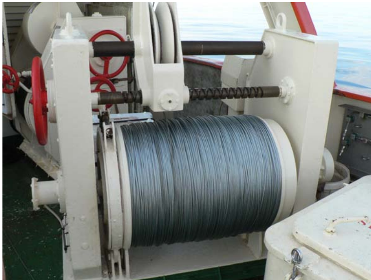
Fig 1. Oceanographic winch on board the Téthys II with a brand-new CTD cable.
